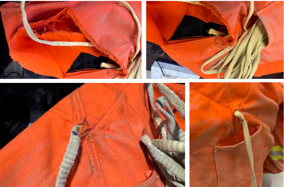
Damage Shown After Repeated Rescue Load Testing
