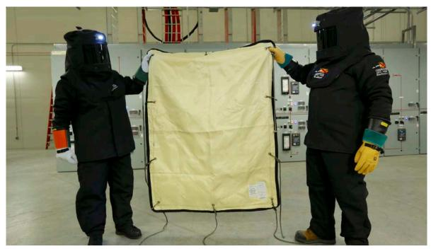
• **Slack vs taut:** By allowing slack when installing the blanket panel, the material can expand and move away from the arc to allow a path for the energy to travel. Loose wrapping can allow energy to shunt out the ends, following the path of least resistance. Arc protective blankets are primarily designed to redirect the arc exposure energy, not to contain. Consider the direction where the arc exposure energy will be directed when designing the installation and determining worker positioning.
