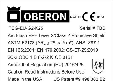
\*Important Note: In addition to the European Standards previously listed, this face shield has also been tested accordance with ASTM F2178-17 and has achieved a determination of ATPV, 50% of probability of the onset of a 2nd degree burn result, of 42 cal/cm². Results are shown in report 2018US0187. This face shield will be marked with an Arc Rating Limit of 25 cal/cm² per ASTM F2178 guidelines.
