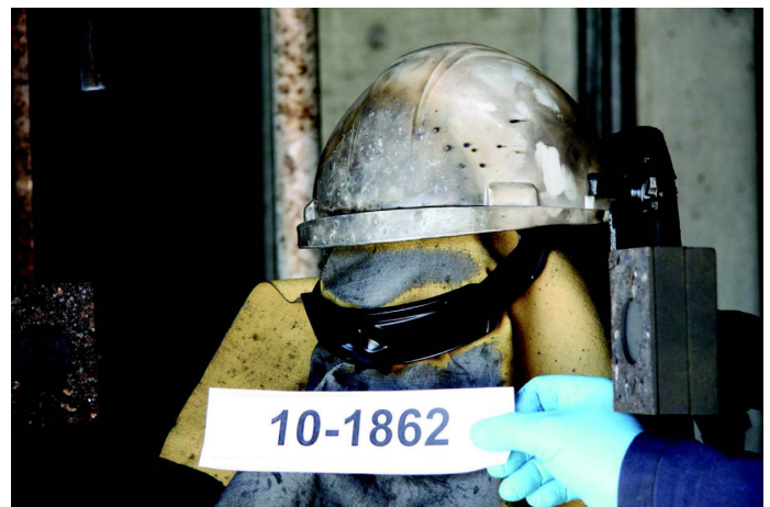
Figure 3: Test 10-1862, Position B after Arc Exposure
